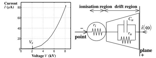
**FIGURE 1.** Current-voltage curve and schematic representation of the point-to-plane loudspeaker.
