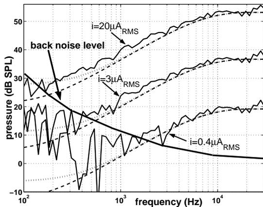
**FIGURE 2.** Frequency responses of the point-to-plane loudspeaker. ( $I = 60\mu A$ ,  $d = 6mm$ ,  $r = 30cm$ ). Theoretical predictions : force source with a cylindrical volume (eq. 4) (---), and with a truncated conical volume (....).
