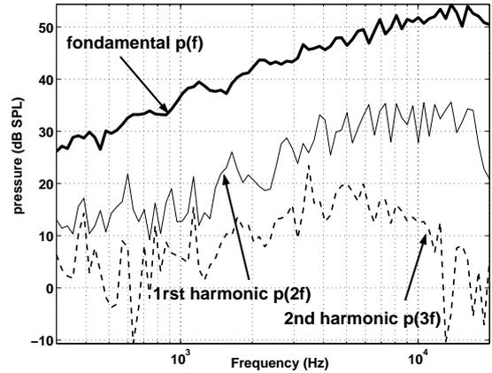
**FIGURE 3.** Sound pressure level of the harmonics ( $I = 60\mu A$ ,  $i = 20\mu A_{RMS}$ ,  $d = 5mm$ ,  $r = 30cm$ ).
